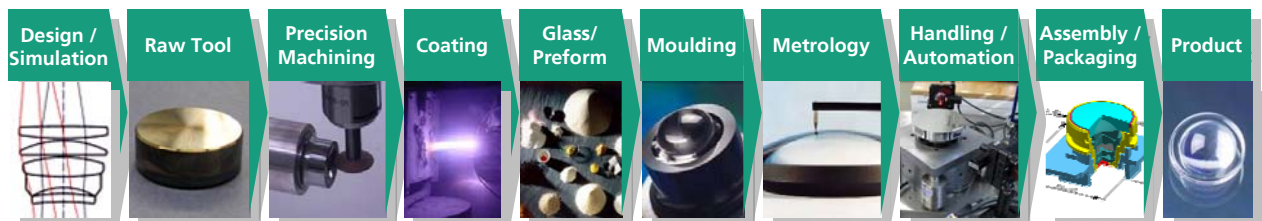
Picture 2: The complete precision glass moulding and mould making process chain
